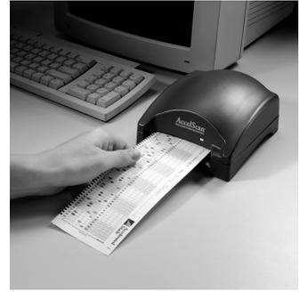
6. After scoring a card, the AccelScan Scanning software will again display the **Ready to scan** message. The scan card will be ejected from the back of the AccelScan.
